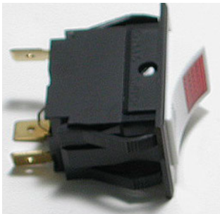
PN: 8573 Switch-Rocker, SPST, On-None-Off, Lit x1
